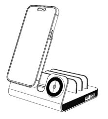
2.2 Charging the watch: Put the watch on the wireless charging area, and align the magnets; the "Charging indicator" on the watch will light up, indicating that it is being charged properly.
