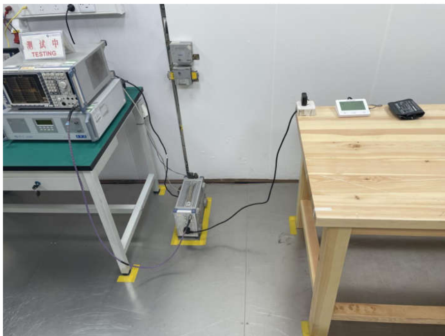
Conducted Emissions Test Setup
