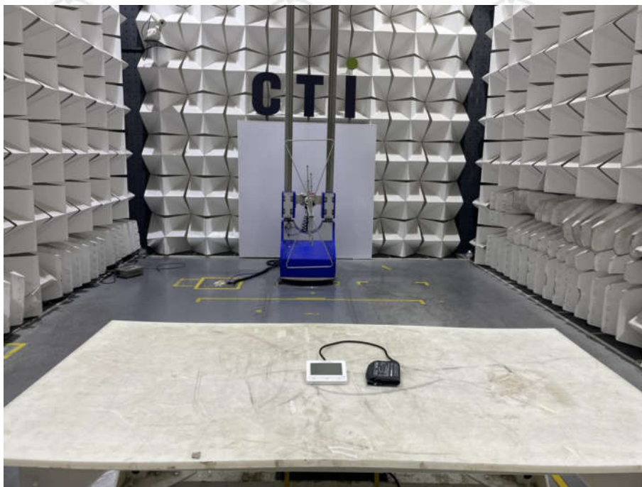
Radiated spurious emission Test Setup-1(Below 1GHz)
