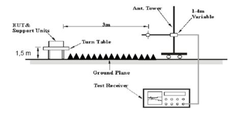
The radiated emission tests were performed in the 3 meters chamber test site, using the setup accordance with the FCC MP - 5. The specification used was the FCC part 18 limits.
