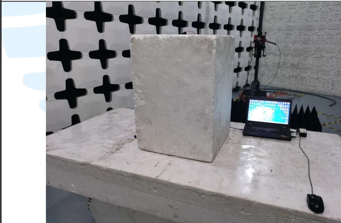
Radiated emission Test Setup (Above 1 GHz) _Right earbuds
