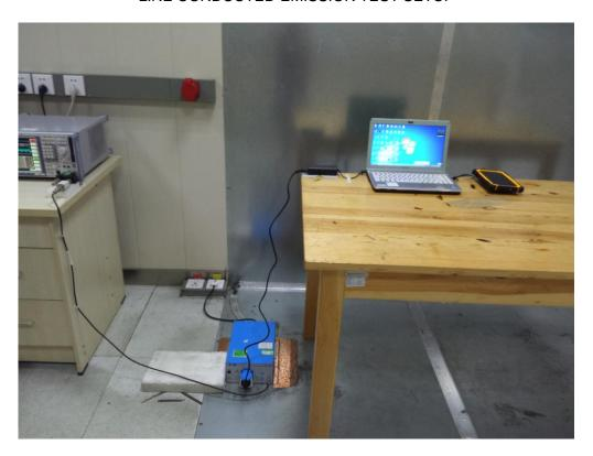
RADIATED EMISSION TEST SETUP
