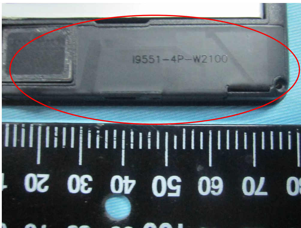
GSM/PCS/UMTS-FDD Antenna View
