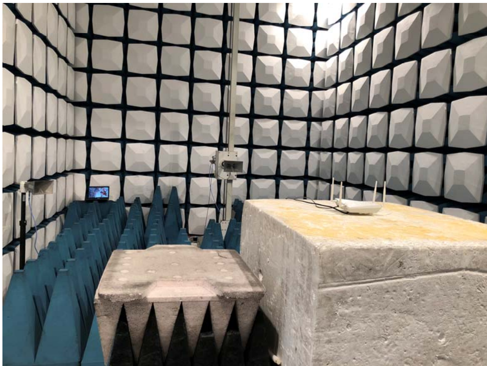
Description: Radiated Emission Test Setup for DFS
