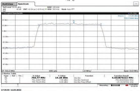
Slot 0 Band 13 (4G LTE) With RP5100 Host, Mod: QPSK, BW: 5 MHz, Ant. Port: ANT1, High Ch. 753.5 MHz 0  $^{\circ}$ C
