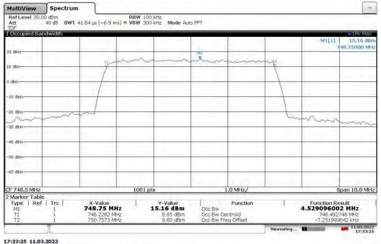
Slot 0 Band 13 (4G LTE) With RP5100 Host, Mod: 64QAM, BW: 5 MHz, Ant. Port: ANT1, Low Ch. 748.5 MHz 0  $^{\circ}$ C
