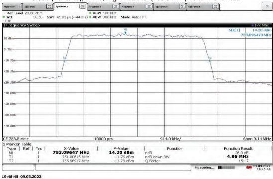
TM3.1a-256QAM\_5 MHz Bandwidth (4G LTE) With RP5100 Host Slot 0 (Band 13), ANT1, High Channel (753.5 MHz) 26 dB Bandwidth
