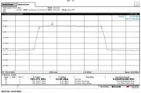
Slot 0 Band 13 (4G LTE) With RP5100 Host, Mod: QPSK, BW: 5 MHz, Ant. Port: ANT1, High Ch. 753.5 MHz 40 °C
