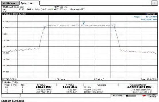
Slot 0 Band 13 (4G LTE) With RP5100 Host, Mod: 64QAM, BW: 5 MHz, Ant. Port: ANT1, Low Ch. 748.5 MHz 40 °C
