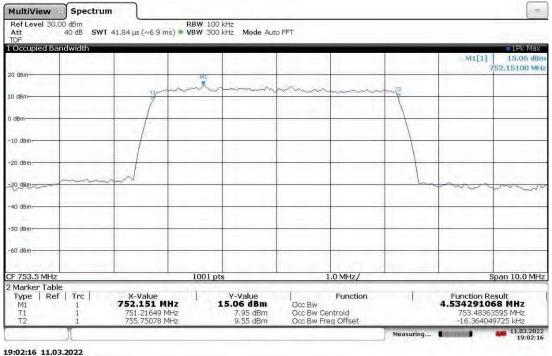
Slot 0 Band 13 (4G LTE) With RP5100 Host, Mod: QPSK, BW: 5 MHz, Ant. Port: ANT1, High Ch. 753.5 MHz 50 °C
