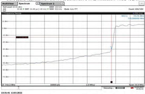
Band Edge Compliant, Lower Band Edge, 748.5 MHz (4G LTE) With RP5100 Host Slot 0 (Band 13), Antenna Port: ANT1, Bandwidth: 5 MHz, Modulation: TM3.2-16QAM
