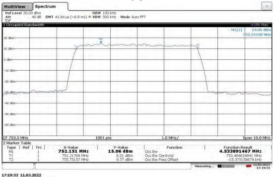
Slot 0 Band 13 (4G LTE) With RP5100 Host, Mod: QPSK, BW: 5 MHz, Ant. Port: ANT1, High Ch. 753.5 MHz 10 °C
