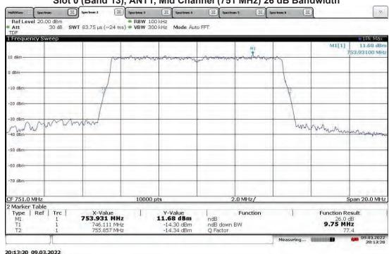
Non-Specific Radio Report Shell Rev. December 2017 Page 61 of 120 Client: CommScope Technologies LLC – Model: RPM-A5A11-B13 with W/ 4G LTE With OneCell® RP5100
