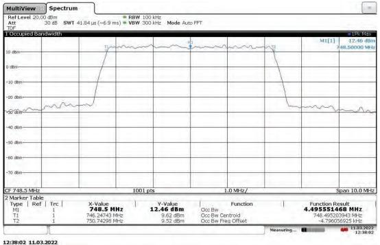
Slot 0 Band 13 (4G LTE) With RP5100 Host, Mod: QPSK, BW: 5 MHz, Ant. Port: ANT1, Low Ch. 748.5 MHz 48 VDC
