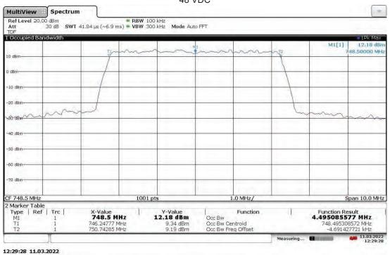
Slot 0 Band 13 (4G LTE) With RP5100 Host, Mod: QPSK, BW: 5 MHz, Ant. Port: ANT1, Low Ch. 748.5 MHz 57 VDC
