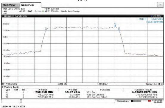
Slot 0 Band 13 (4G LTE) With RP5100 Host, Mod: 64QAM, BW: 5 MHz, Ant. Port: ANT1, Low Ch. 748.5 MHz 30  $^{\circ}$ C
