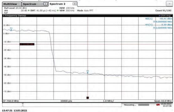
Band Edge Compliant, Upper Band Edge, 753.5 MHz (4G LTE) With RP5100 Host Slot 0 (Band 13), Antenna Port: ANT1, Bandwidth: 5 MHz, Modulation: TM1.1-QPSK
