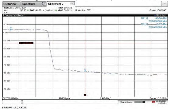
Band Edge Compliant, Upper Band Edge, 753.5 MHz (4G LTE) With RP5100 Host Slot 0 (Band 13), Antenna Port: ANT1, Bandwidth: 5 MHz, Modulation: TM3.1-64QAM
