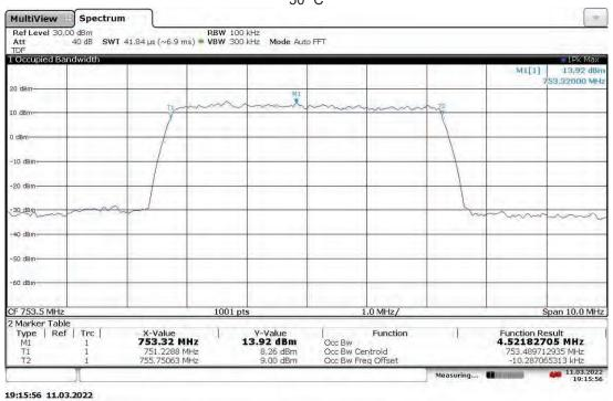
Slot 0 Band 13 (4G LTE) With RP5100 Host, Mod: QPSK, BW: 5 MHz, Ant. Port: ANT1, Low Ch. 748.5 MHz 41.1 VDC
