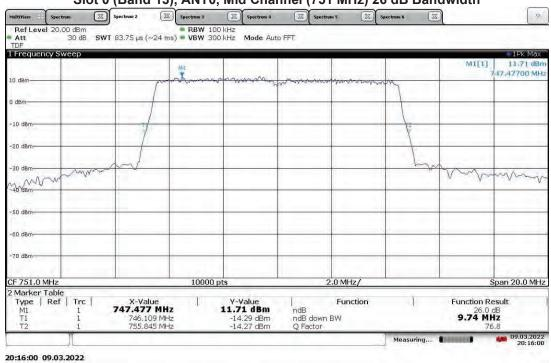
TM1.1-QPSK\_10 MHz Bandwidth (4G LTE) With RP5100 Host Slot 0 (Band 13), ANT1, Mid Channel (751 MHz) 26 dB Bandwidth
