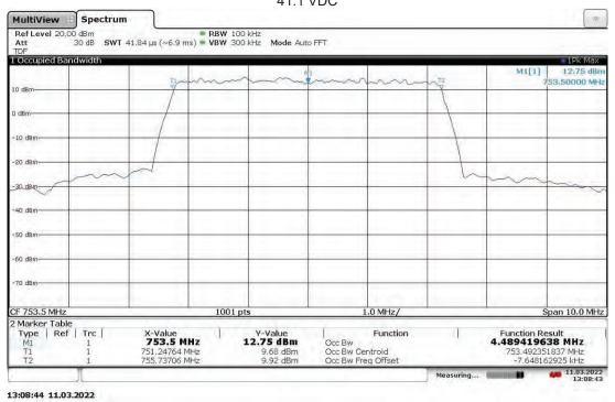
Slot 0 Band 13 (4G LTE) With RP5100 Host, Mod: QPSK, BW: 5 MHz, Ant. Port: ANT1, High Ch. 753.5 MHz 48 VDC
