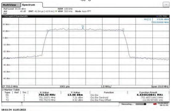
Slot 0 Band 13 (4G LTE) With RP5100 Host, Mod: QPSK, BW: 5 MHz, Ant. Port: ANT1, High Ch. 753.5 MHz -20 °C
