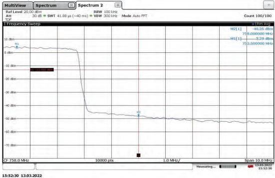
Band Edge Compliant, Upper Band Edge, 753.5 MHz (4G LTE) With RP5100 Host Slot 0 (Band 13), Antenna Port: ANT1, Bandwidth: 5 MHz, Modulation: TM3.1a-256QAM
