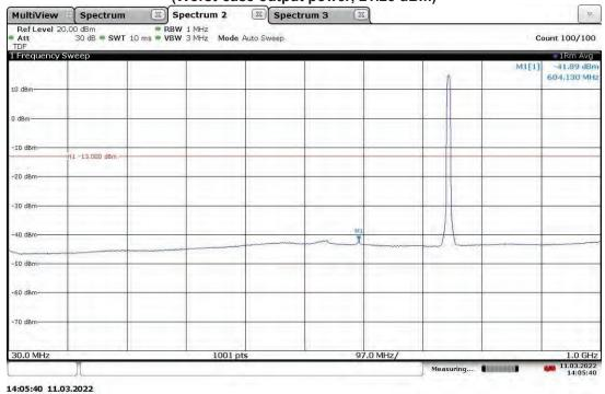
Antenna Port (ANT1) Conducted Emissions, 1-8 GHz Band 13 (4G LTE), Mid Channel 751 MHz, BW 5 MHz, Modulation QPSK (Worst-case output power, 21.25 dBm)
