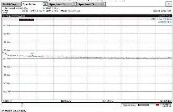
Antenna Port (ANT0) Conducted Emissions, 30 MHz-1 GHz Band 13 (4G LTE), Mid Channel 751 MHz, BW 5 MHz, Modulation QPSK (Worst-case output power, 21.25 dBm)
