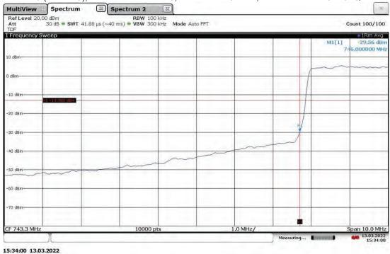
Band Edge Compliant, Lower Band Edge, 748.5 MHz (4G LTE) With RP5100 Host Slot 0 (Band 13), Antenna Port: ANT1, Bandwidth: 5 MHz, Modulation: TM3.1-64QAM
