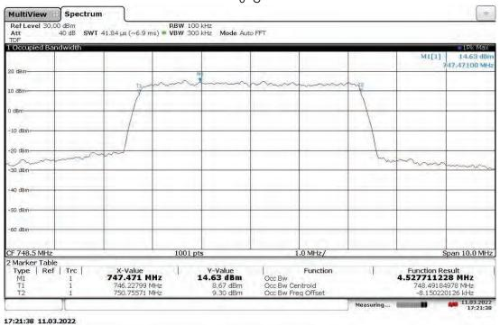
Slot 0 Band 13 (4G LTE) With RP5100 Host, Mod: 64QAM, BW: 5 MHz, Ant. Port: ANT1, Low Ch. 748.5 MHz 10 °C
