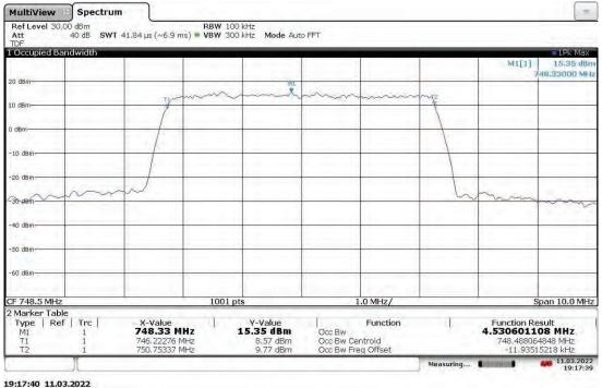
Slot 0 Band 13 (4G LTE) With RP5100 Host, Mod: QPSK, BW: 5 MHz, Ant. Port: ANT1, High Ch. 753.5 MHz -30 °C
