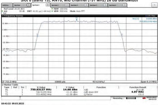
TM3.1-64QAM\_5 MHz Bandwidth (4G LTE) With RP5100 Host Slot 0 (Band 13), ANT1, Mid Channel (751 MHz) 26 dB Bandwidth
