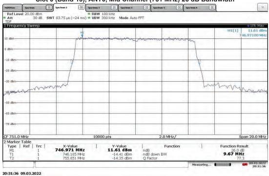
TM3.1-64QAM\_10 MHz Bandwidth (4G LTE) With RP5100 Host Slot 0 (Band 13), ANT1, Mid Channel (751 MHz) Occupied Bandwidth
