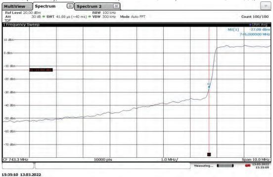
Band Edge Compliant, Lower Band Edge, 748.5 MHz (4G LTE) With RP5100 Host Slot 0 (Band 13), Antenna Port: ANT1, Bandwidth: 5 MHz, Modulation: TM3.1a-256QAM
