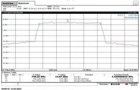
Slot 0 Band 13 (4G LTE) With RP5100 Host, Mod: 64QAM, BW: 5 MHz, Ant. Port: ANT1, Low Ch. 748.5 MHz -20 °C
