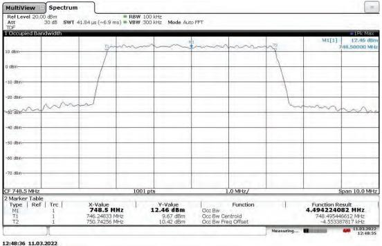
Slot 0 Band 13 (4G LTE) With RP5100 Host, Mod: QPSK, BW: 5 MHz, Ant. Port: ANT1, High Ch. 753.5 MHz 41.1 VDC
