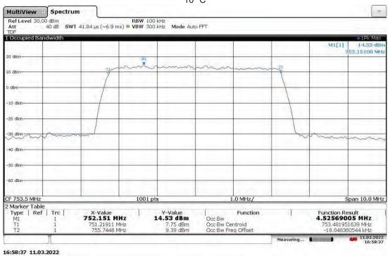
Slot 0 Band 13 (4G LTE) With RP5100 Host, Mod: QPSK, BW: 5 MHz, Ant. Port: ANT1, High Ch. 753.5 MHz 20 °C
