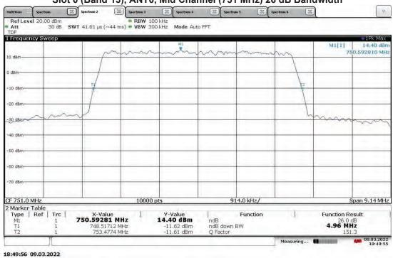
TM3.1a-256QAM\_5 MHz Bandwidth (4G LTE) With RP5100 Host Slot 0 (Band 13), ANT1, Mid Channel (751 MHz) 26 dB Bandwidth
