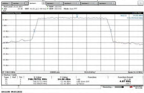
TM3.1a-256QAM\_5 MHz Bandwidth (4G LTE) With RP5100 Host Slot 0 (Band 13), ANT1, Low Channel (748.5 MHz) 26 dB Bandwidth
