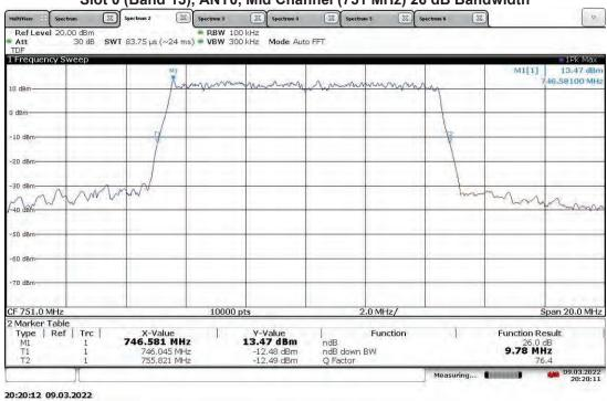
TM3.2-16QAM\_10 MHz Bandwidth (4G LTE) With RP5100 Host Slot 0 (Band 13), ANT1, Mid Channel (751 MHz) 26 dB Bandwidth
