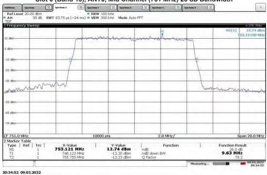
TM3.1a-256QAM\_10 MHz Bandwidth (4G LTE) With RP5100 Host Slot 0 (Band 13), ANT1, Mid Channel (751 MHz) 26 dB Bandwidth
