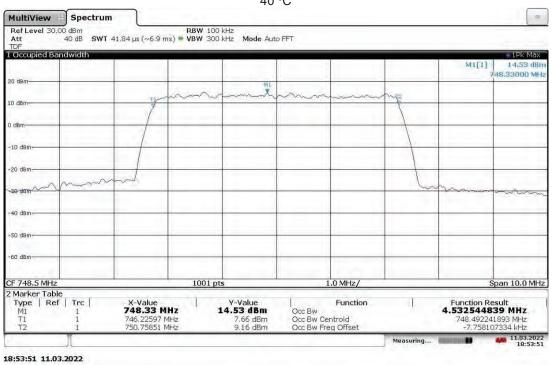
Slot 0 Band 13 (4G LTE) With RP5100 Host, Mod: 64QAM, BW: 5 MHz, Ant. Port: ANT1, Low Ch. 748.5 MHz 50  $^{\circ}$ C
