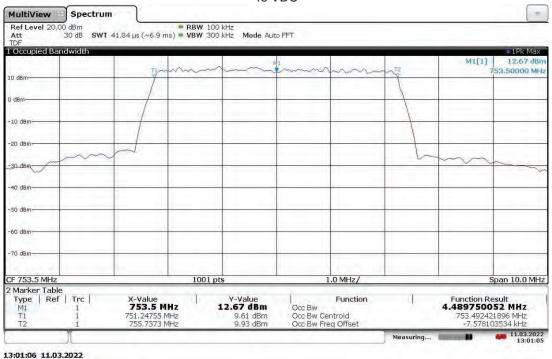
Slot 0 Band 13 (4G LTE) With RP5100 Host, Mod: QPSK, BW: 5 MHz, Ant. Port: ANT1, High Ch. 753.5 MHz 57 VDC
