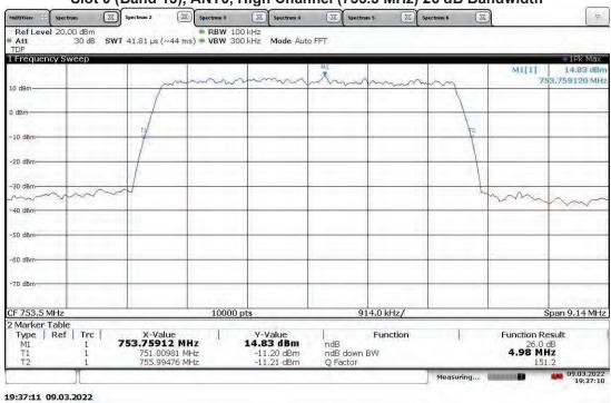
TM3.1-64QAM\_5 MHz Bandwidth (4G LTE) With RP5100 Host Slot 0 (Band 13), ANT1, High Channel (753.5 MHz) 26 dB Bandwidth
