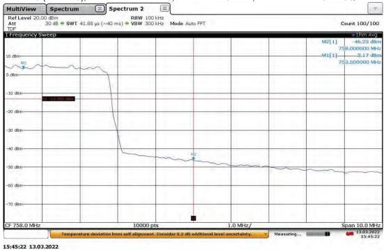
Band Edge Compliant, Upper Band Edge, 753.5MHz (4G LTE) With RP5100 Host Slot 0 (Band 13), Antenna Port: ANT1, Bandwidth: 5 MHz, Modulation: TM3.2-16QAM
