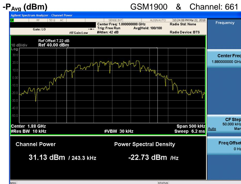
$$\text{PAPR (dB)} = \text{P}_{\text{Pk}} (\text{dBm}) - \text{P}_{\text{Avg}} (\text{dBm}) = 31.61 \text{ dBm} - 31.13 \text{ dBm} = 0.48 \text{ dB}$$
