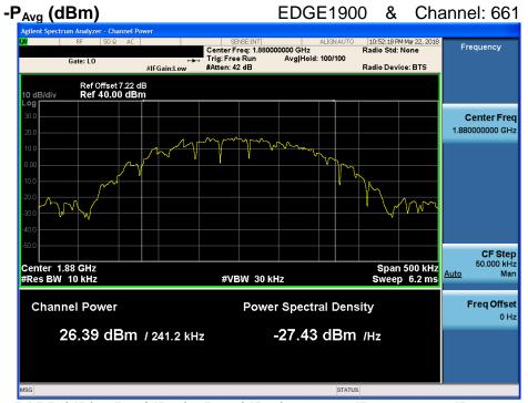
$PAPR(dB) = P_{Pk}(dBm) - P_{Avg}(dBm) = 30.05 dBm - 26.39 dBm = 3.66 dB$
