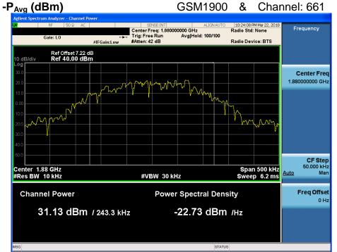
PAPR (dB) =  $P_{Pk}$  (dBm) -  $P_{Avg}$  (dBm) = 31.61 dBm - 31.13 dBm = 0.48 dB
