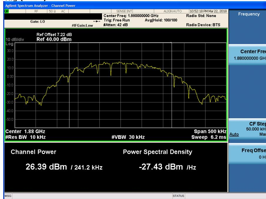
$$PAPR (dB) = P_{Pk} (dBm) - P_{Avg} (dBm) = 30.05 \text{ dBm} - 26.39 \text{ dBm} = 3.66 \text{ dB}$$
