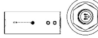
3.8. Screw the sight glass back into the gauge and tighten by hand.
