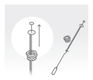
**e.** Remove the steel wire assembly from the bushing by gently pulling it upward while holding the bushing.
