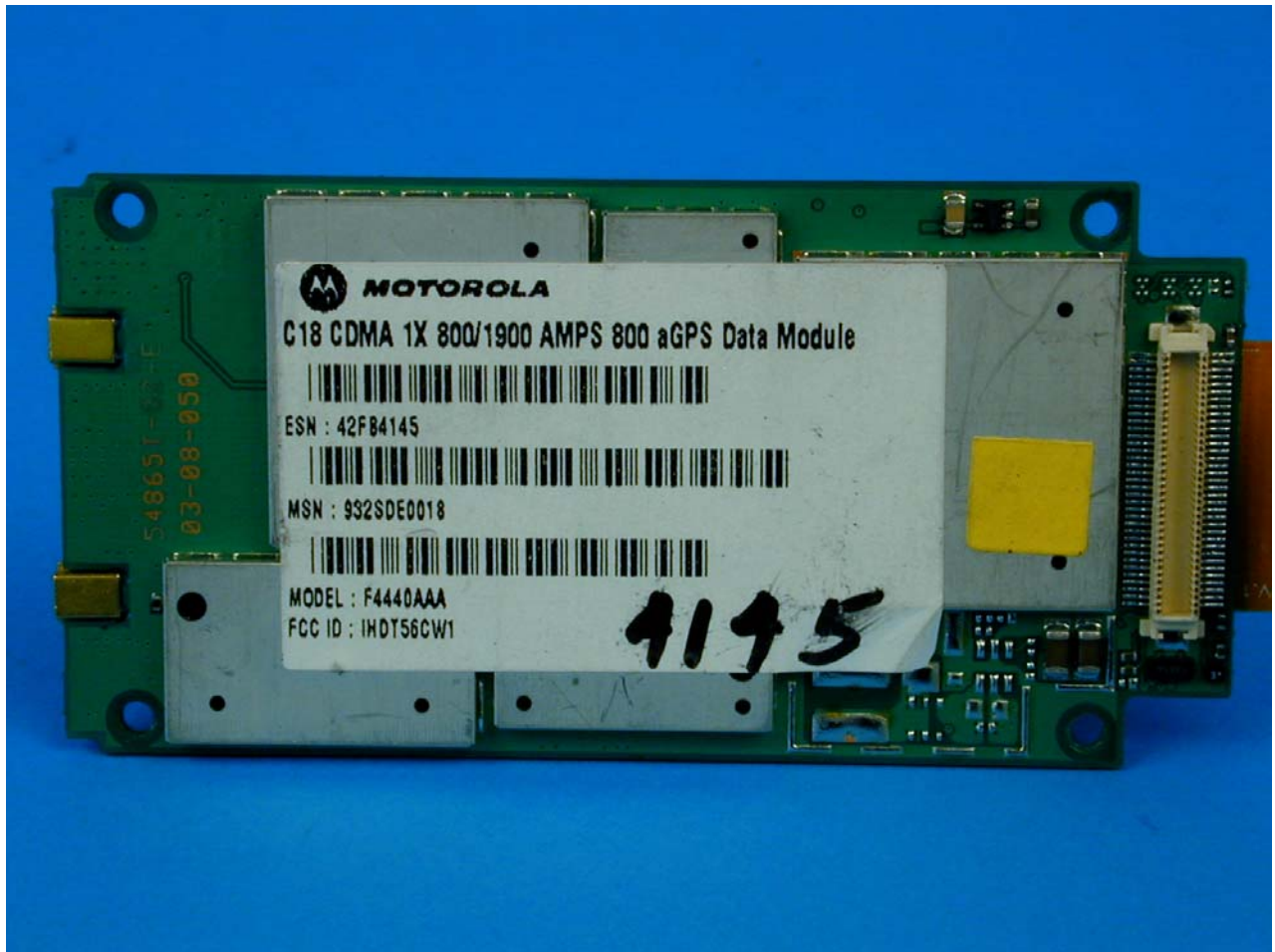
Photograph 11 4111-CDMA Front View of C18 CDMA Module
