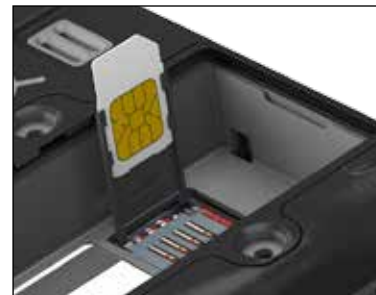
Installing the SIM Card
