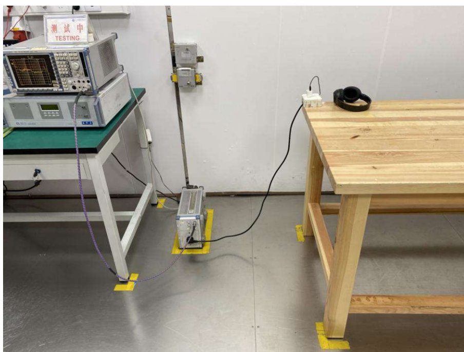
AC Power Line Conducted Emission
