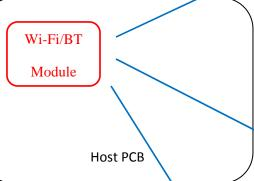
Since the module size is too small, when installed into the host, an additional permanent label referring to the enclosed module: "Contains FCC ID: JUP-95807WFBT, IC: 1756A-95807WFBT" must be used.
