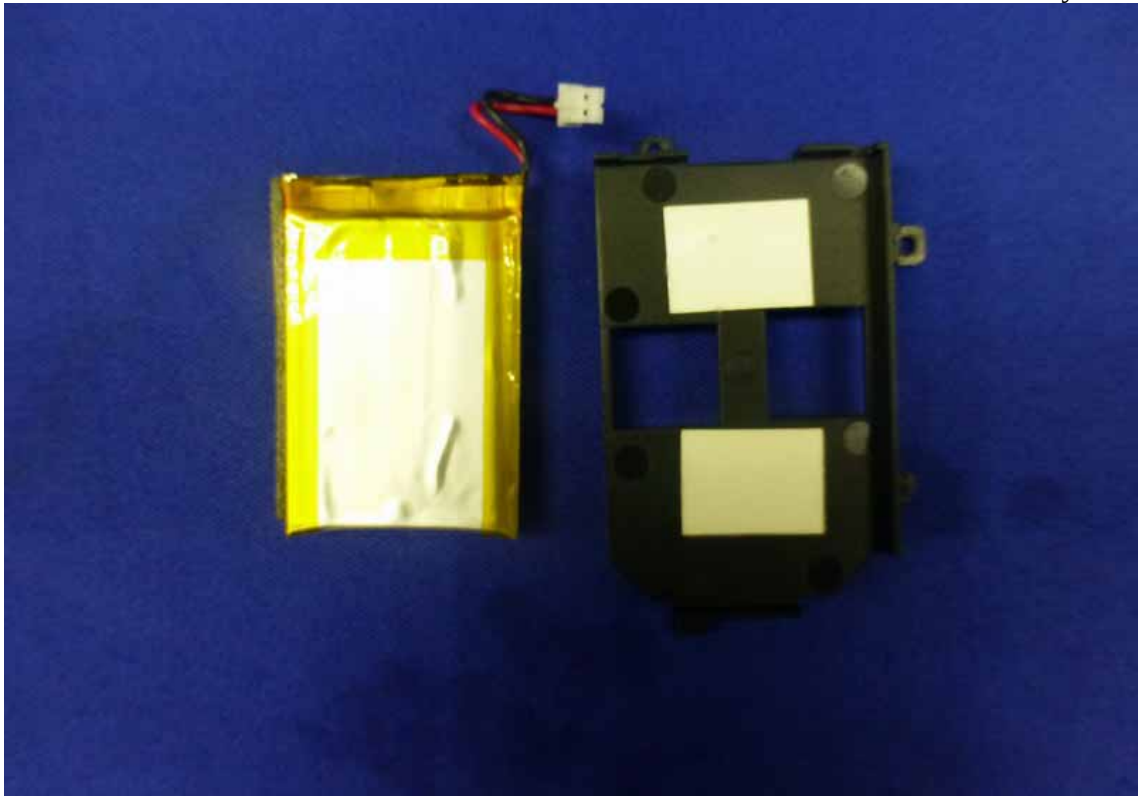
Figure 15 Battery of the EUT
