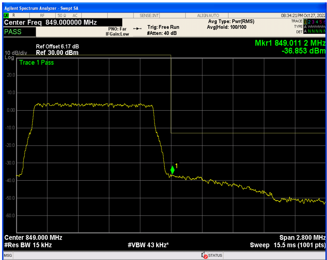
Band5 QAM16 BW=1.4MHz Channel=20643 RB Size=1 Position=#Max
