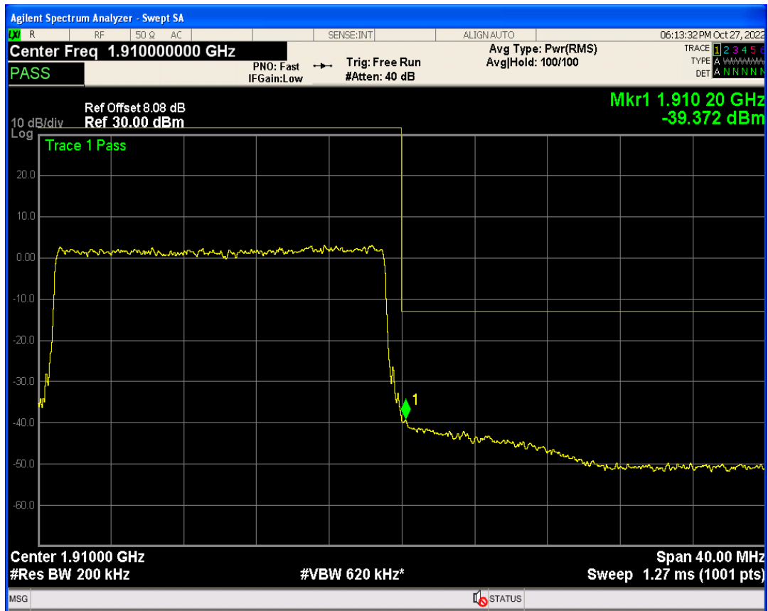
Band2 QAM16 BW=20MHz Channel=19100 RB Size=1 Position=#0
