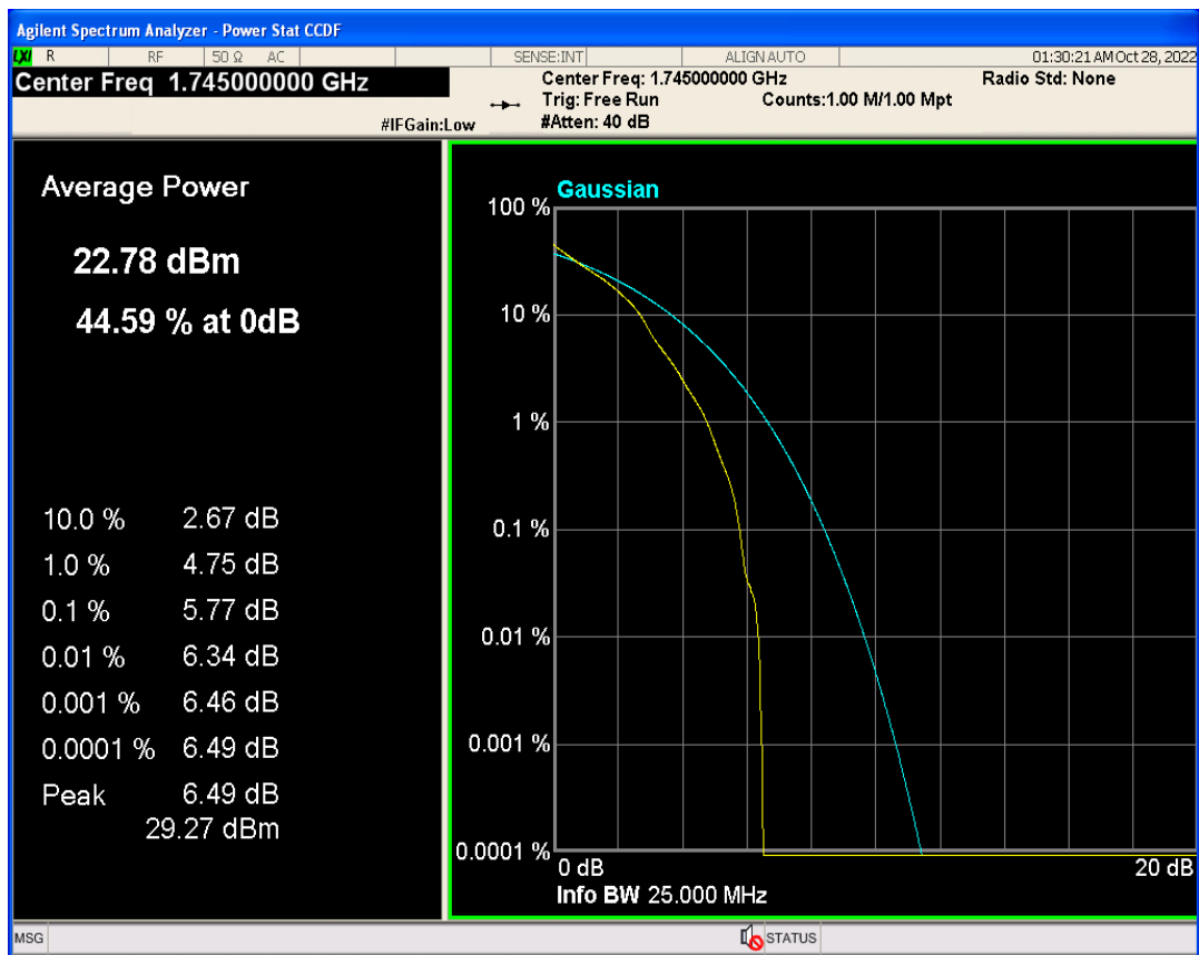
Band66 QAM16 BW=15MHz Channel=132322 RB Size=1 Position=#0
