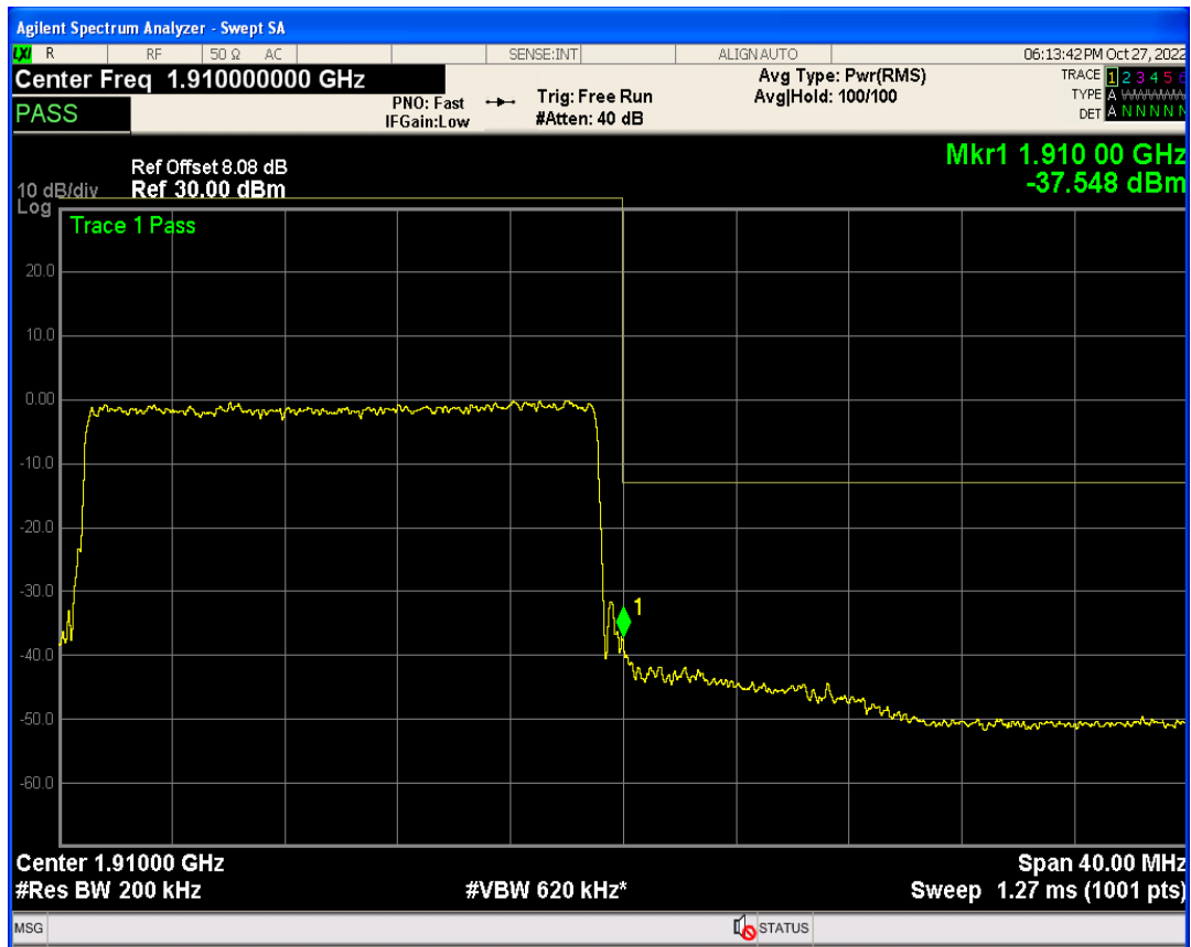
Band2 QAM16 BW=20MHz Channel=19100 RB Size=1 Position=#Max
