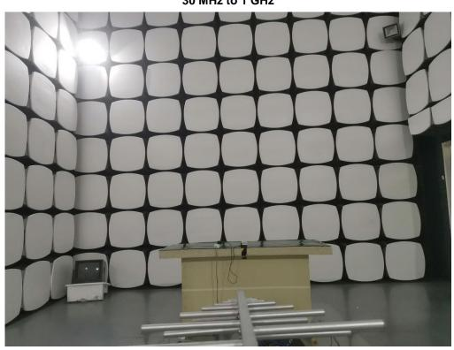
Radiated Emissions Test Photos 30 MHz to 1 GHz
