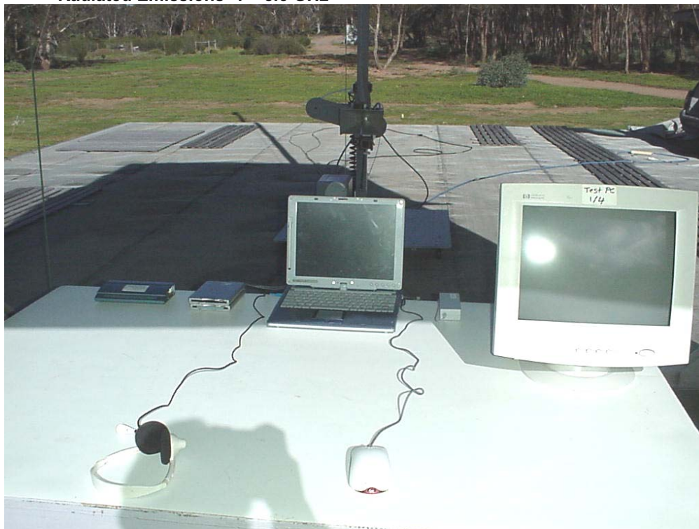
Radiated Emissions 1 – 8.5 GHz
