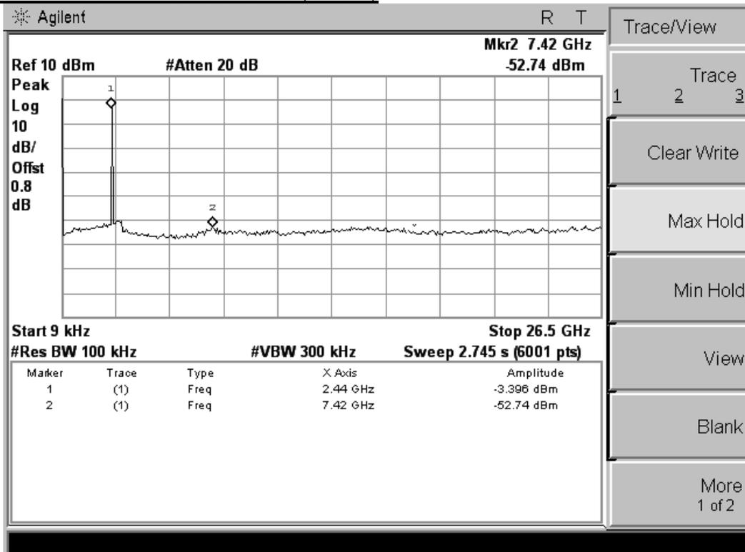
**9KHz-26.5GHz High Channel(GFSK)**
