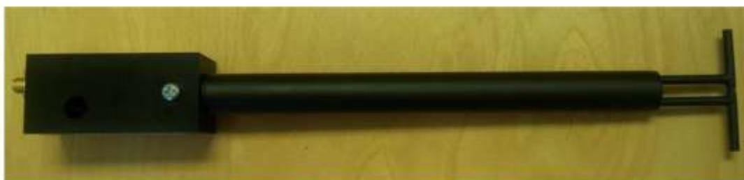
Figure 1 – MVG COMOSAR Validation Dipole
