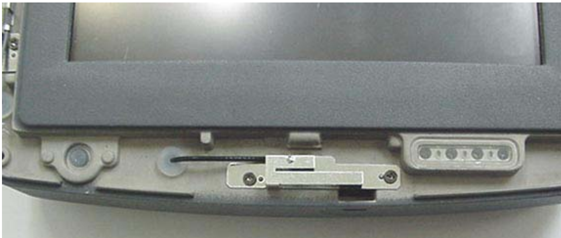
Internal Bluetooth PIFA Antenna
