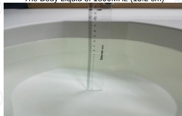
The Body Liquid of 2450MHz (15.3cm)
