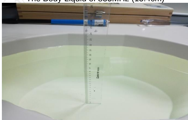
The Body Liquid of 1900MHz (16.4 cm)
