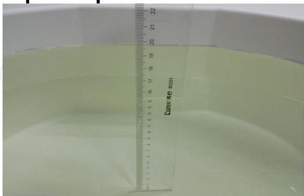
The Body Liquid of 835MHz (15.4cm)
