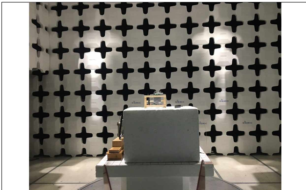
Radiated Emission Test above 1GHz Front View
