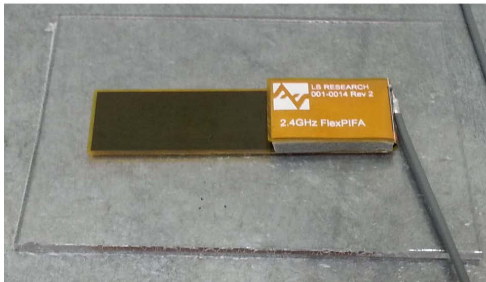
Figure 28 FlexPIFA Mounted on Metal Surface with 1.5mm Thick Polycarbonate Spacer
