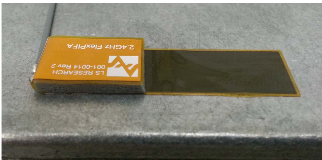
Figure 27 FlexPIFA Mounted on Metal
