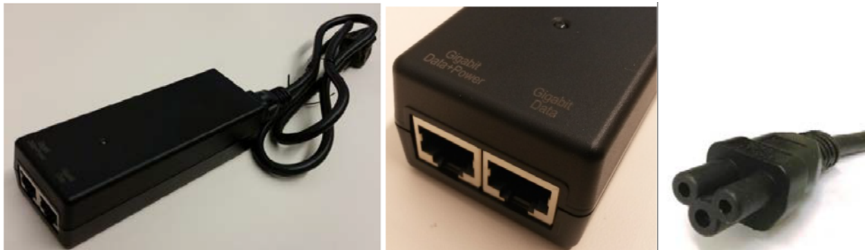
Figure 14 Gigabit Enet Capable power supply
