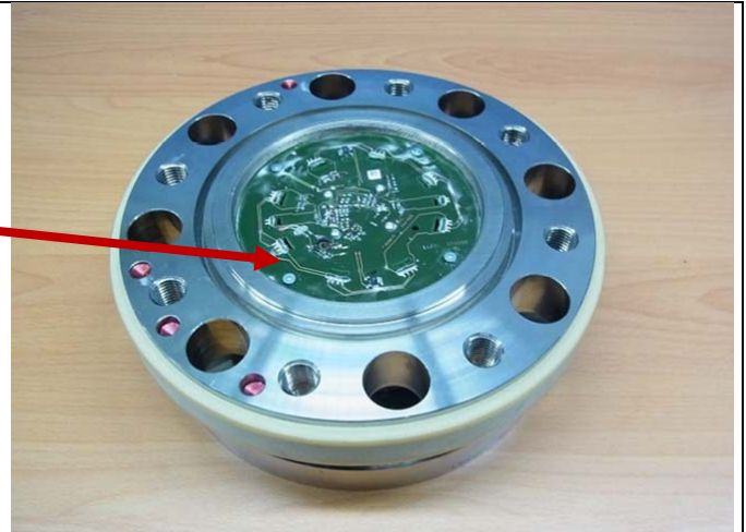
The rotor includes 4 PCB*
