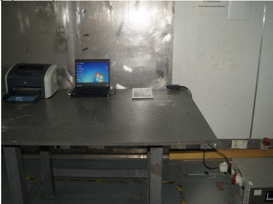
Photograph 2: Set-up for Spurious Emissions below 30MHz
