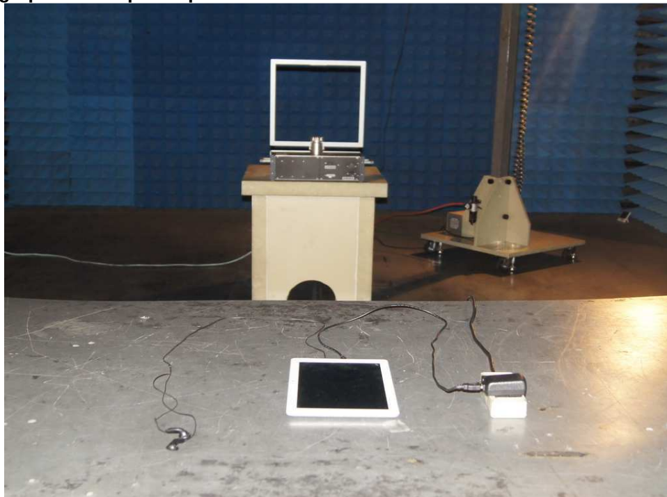
Photograph 2: Set-up for Spurious Emissions below 30MHz
