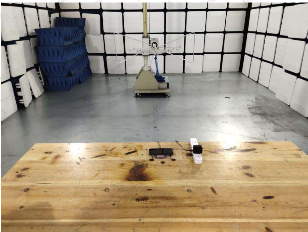
Photo of Radiation Emission Test
