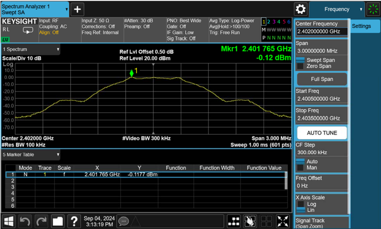
Figure 10: Conducted Spurious Emission & Authorized-band band-edge, 2402MHz, BLE Carrier Level
