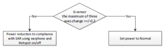
When the maximum of three axes change <+/-0.2, the user case MUST be mobile phone stay away from the body, but if it is>+/-0.2, it MAY be on the person's body, power reduction is on.
