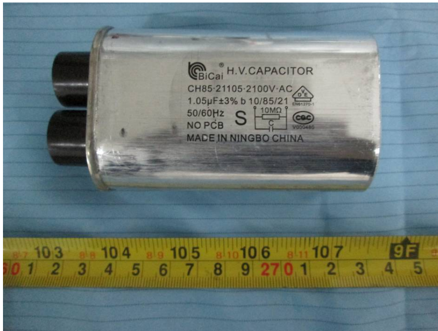
EUT – H.V. Capacitor View
