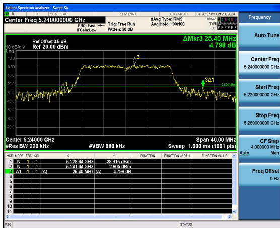
(802.11 a) 26dB Bandwidth plot on channel 48
