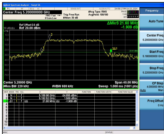
(802.11ac20) 26dB Bandwidth plot on channel 40
