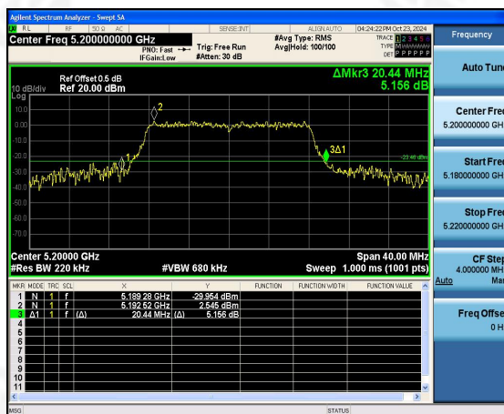
(802.11 a) 26dB Bandwidth plot on channel 40
