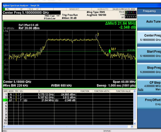
(802.11 a) 26dB Bandwidth plot on channel 36
