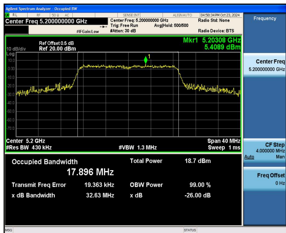
(802.11ac20) 99% Bandwidth plot on channel 40
