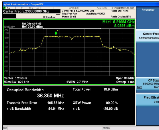
(802.11 n40) 99% Bandwidth plot on channel 46
