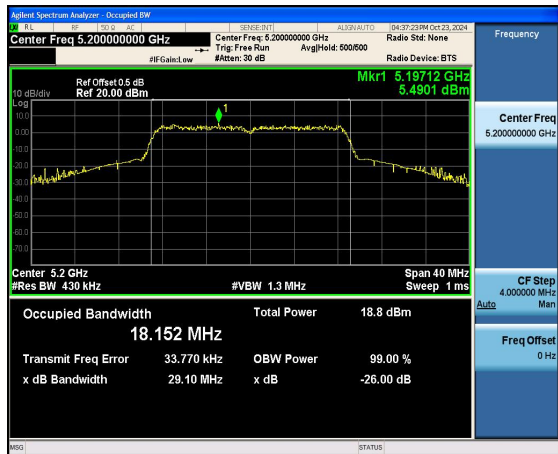
(802.11 n20) 99% Bandwidth plot on channel 48
