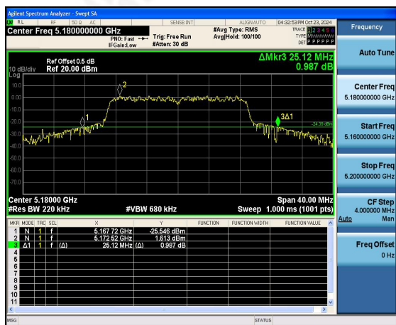
(802.11 n20) 26dB Bandwidth plot on channel 40
