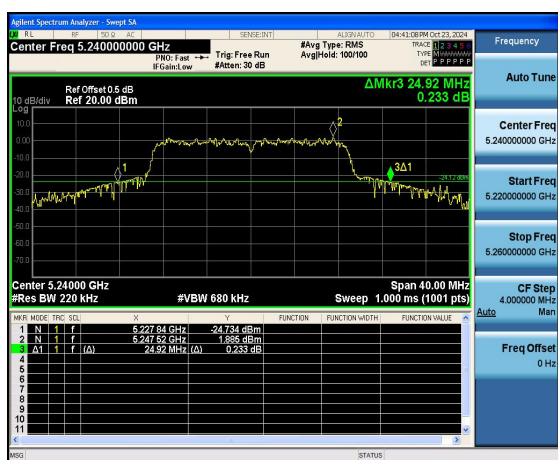
(802.11 n20) 26dB Bandwidth plot on channel 48
