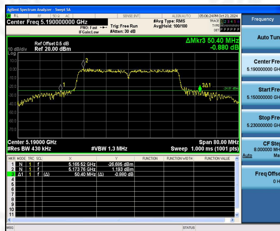
(802.11 ac40) 26dB Bandwidth plot on channel 46
