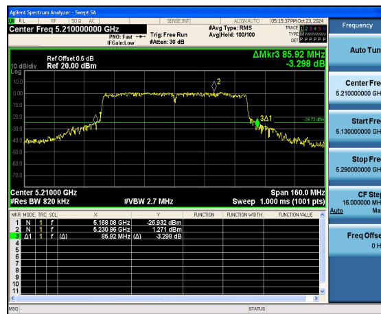
(802.11 ac80) 26dB Bandwidth plot on channel 42
