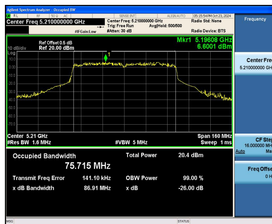
(802.11 ac80) 99% Bandwidth plot on channel 42
