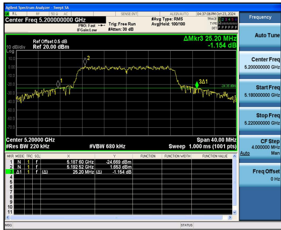
(802.11 n20) 26dB Bandwidth plot on channel 48
