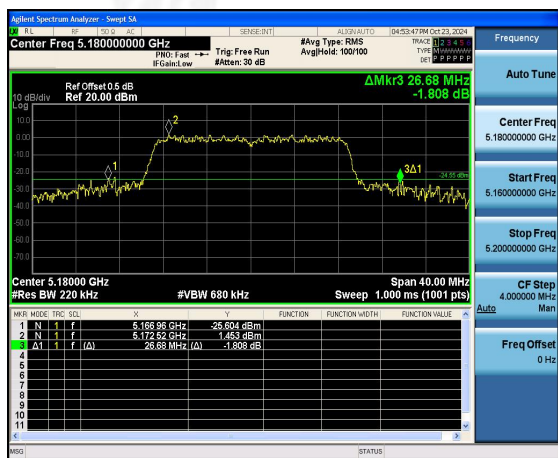
(802.11ac20) 26dB Bandwidth plot on channel 40
