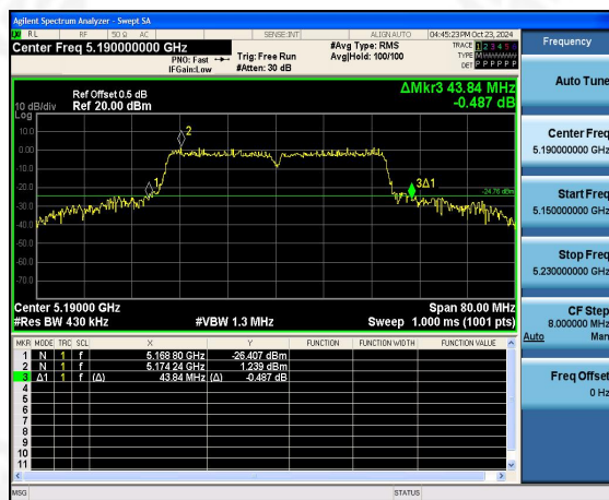
(802.11 n40) 26dB Bandwidth plot on channel 46
