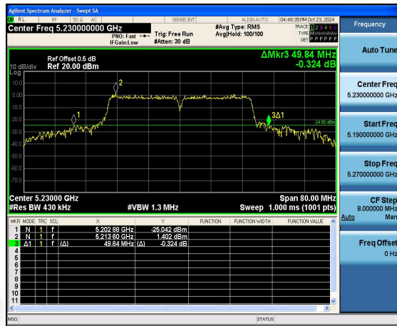
(802.11 n40) 26dB Bandwidth plot on channel 46
