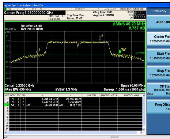
(802.11 ac40) 26dB Bandwidth plot on channel 46
