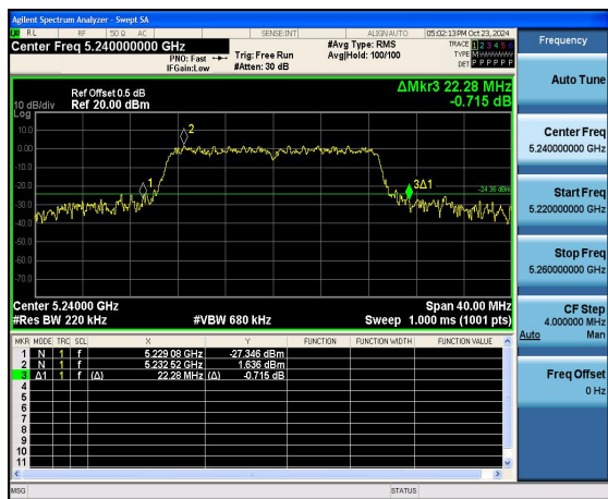
(802.11ac20) 26dB Bandwidth plot on channel 48
