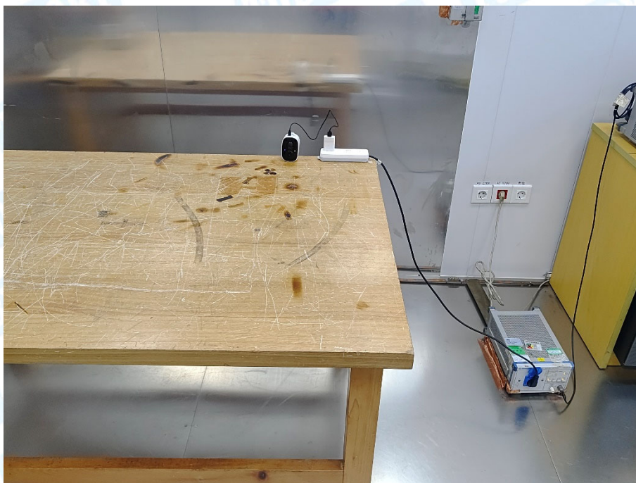
Photo of Setup for Conducted Emission
