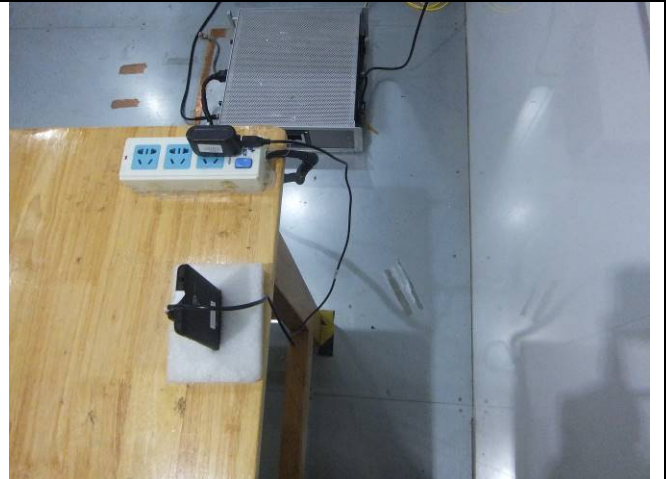
Conducted Emissions Test Setup Side View
