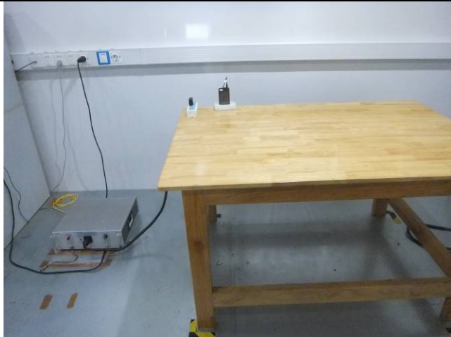
Conducted Emissions Test Setup Front View
