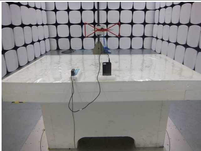
Conducted Emissions Test Setup Front View
