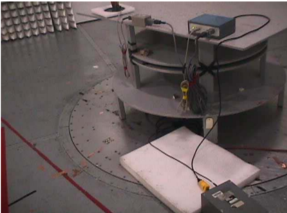
Conducted Emissions Test Configuration
