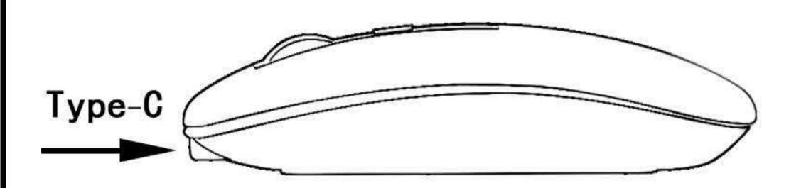
Charging cable connected to the computer is USB, charging when the red light, the charging process is about 1-2 hours, charging complete the red light goes ot
