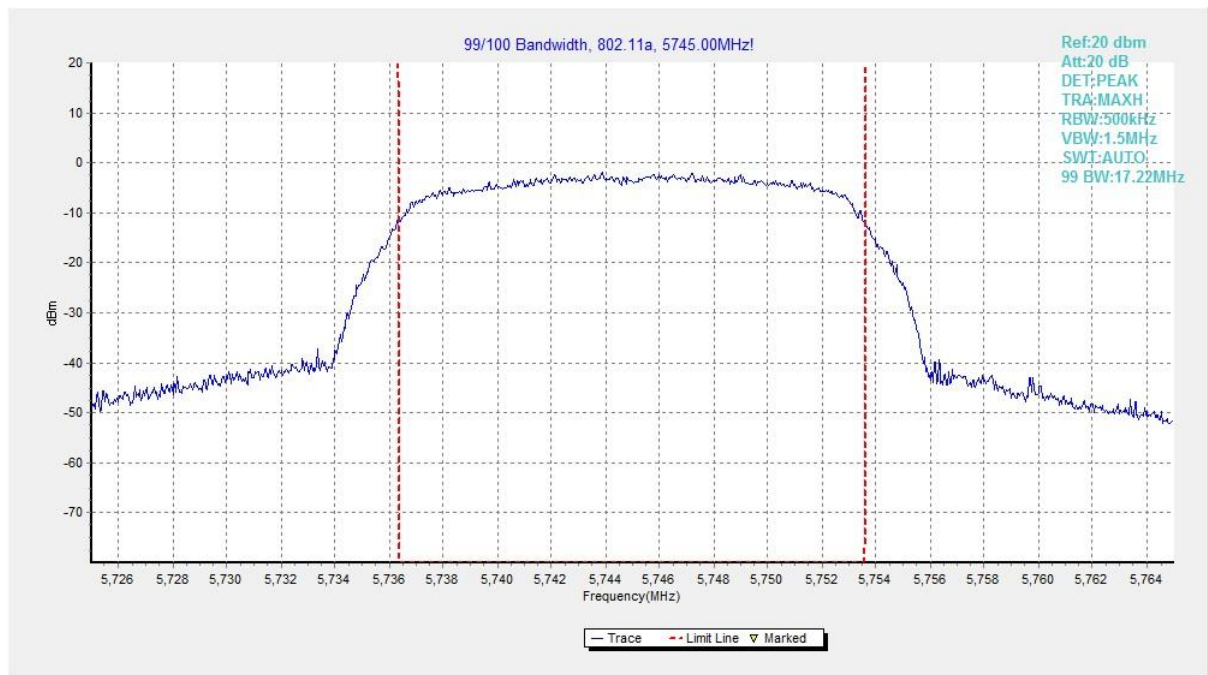
Fig. 25 99% Occupied Bandwidth (802.11a, 5745MHz)
