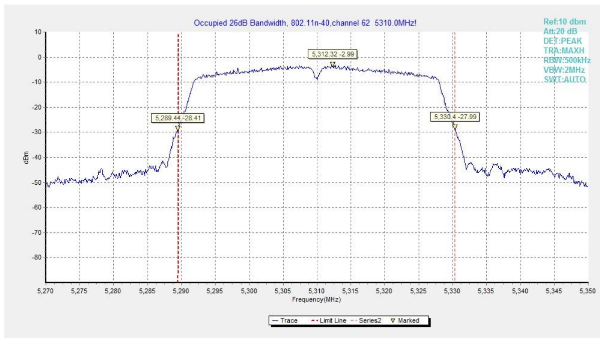
Fig. 10 Occupied 26dB Bandwidth (802.11n-HT40, 5310MHz)
