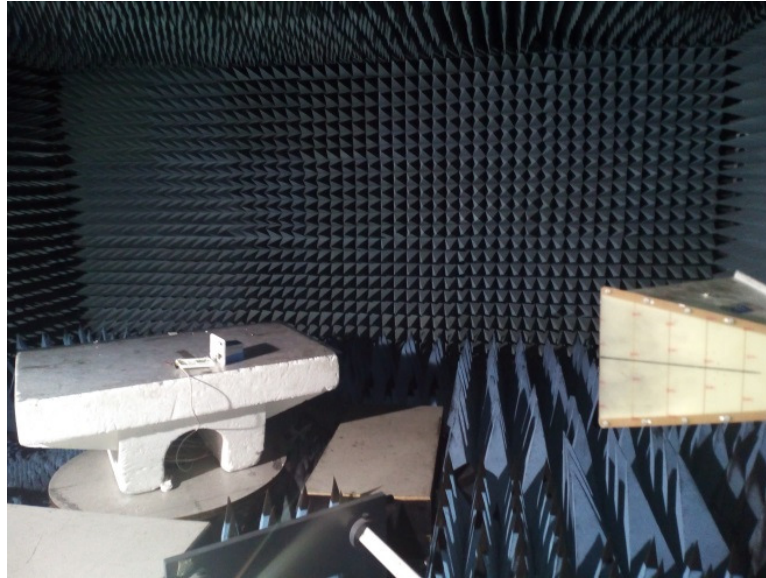
Photograph 8.1.2 Setup for radiated emission measurements
