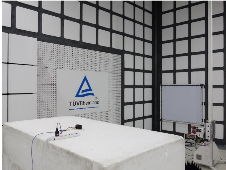
Photograph 5: Test Setup for Spurious Emissions (Back View 3)
