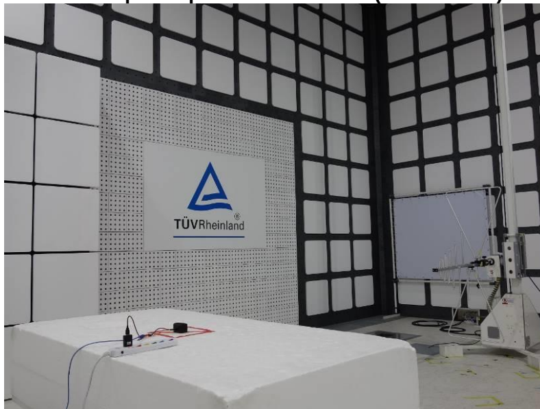
Photograph 4: Test Setup for Spurious Emissions (Back View 2)
