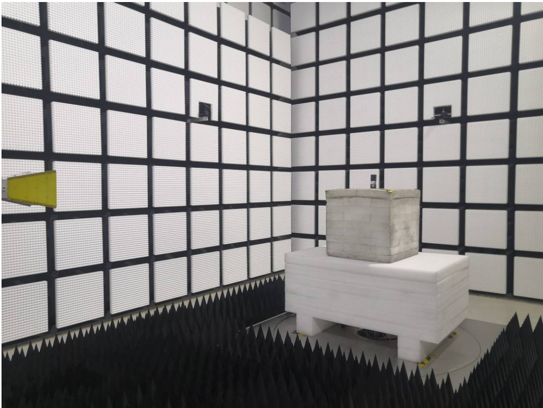
Radiated Emissions Above 1G View Adapter 1#
