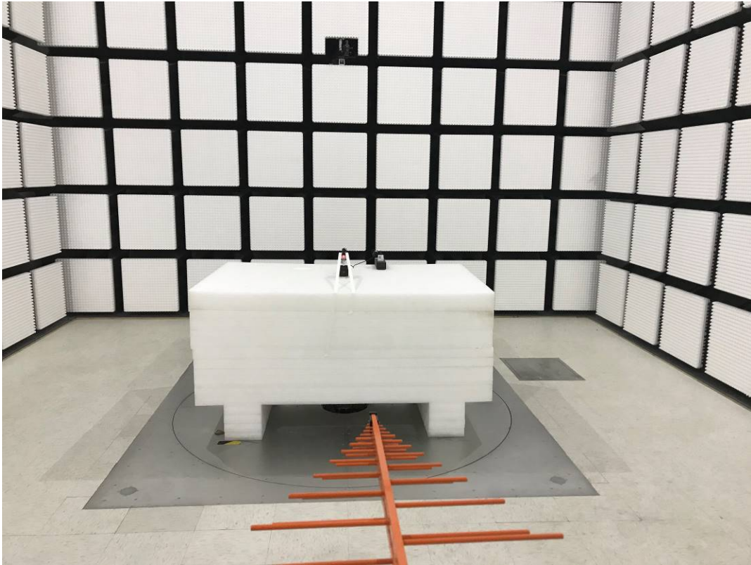
Radiated Emissions Below 1G View Adapter 1#
