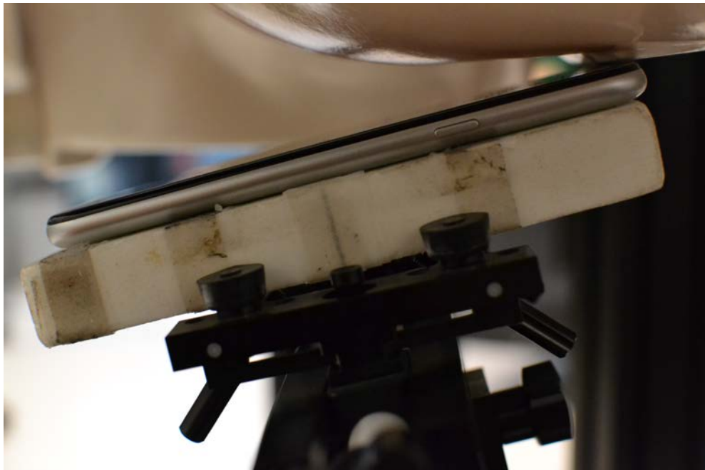
SAR Test Setup Photo 2: Left Tilt
