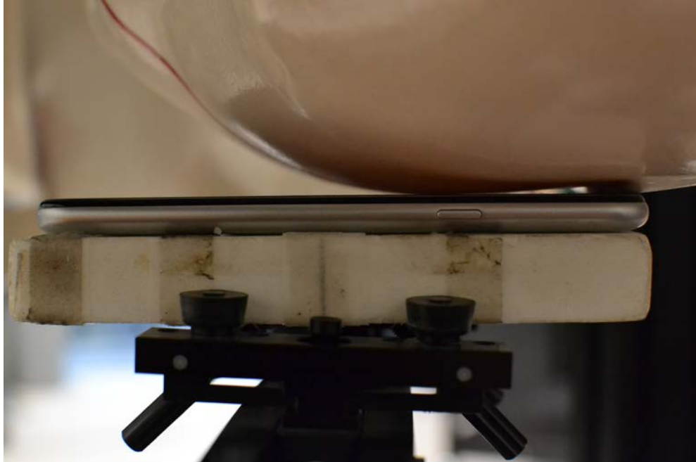
SAR Test Setup Photo 1: Left Cheek
