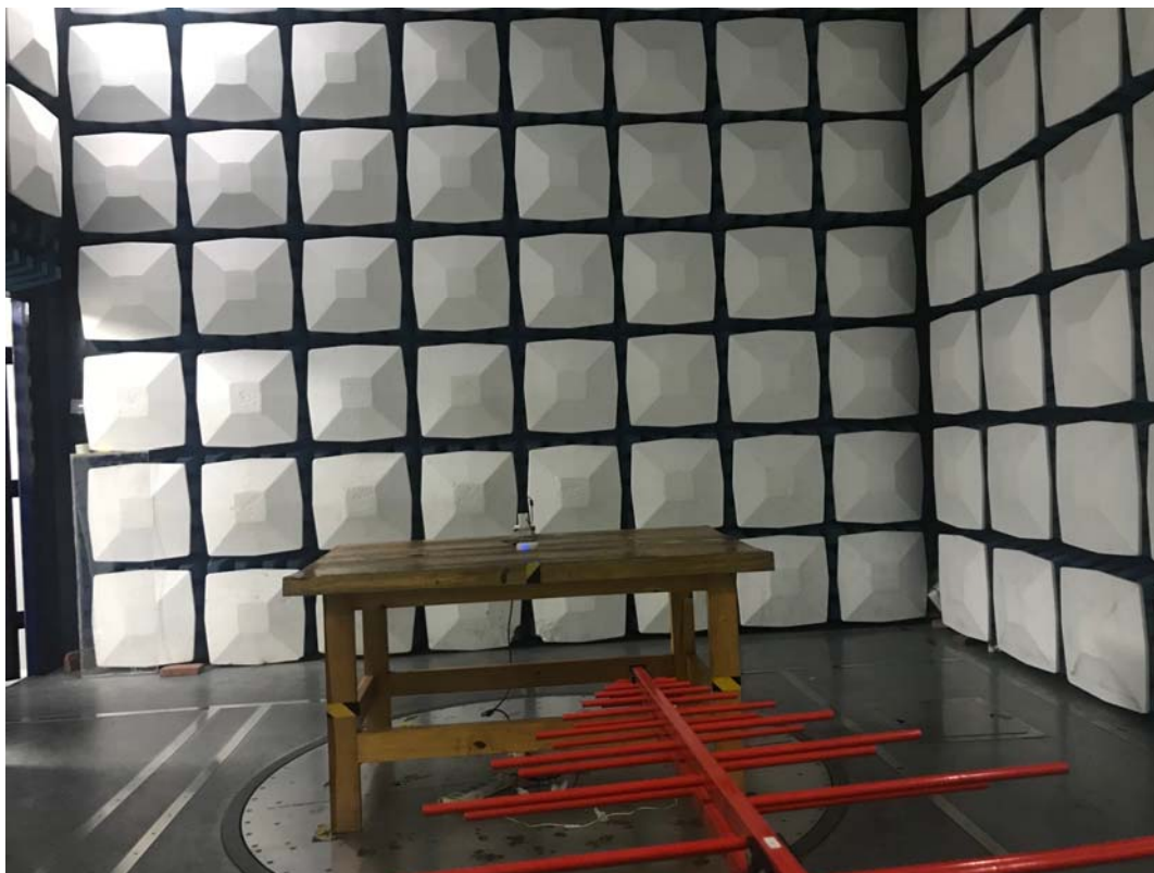
Radiated Emission Above 1GHz View
