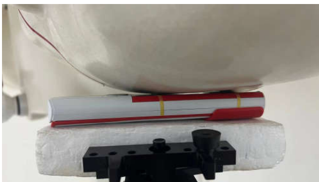
Left Cheek, Test Separation 0 mm
