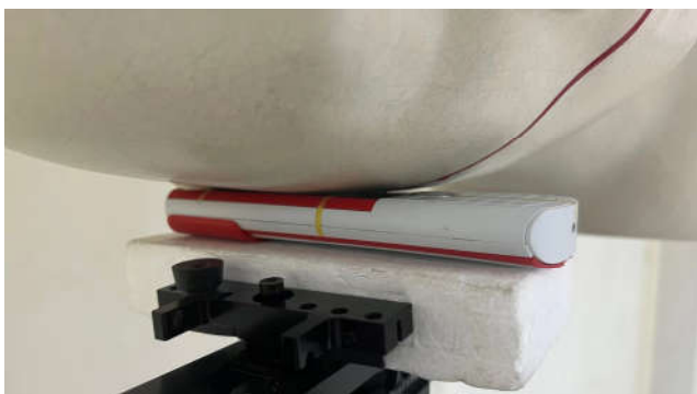
Right Cheek, Test Separation 0 mm
