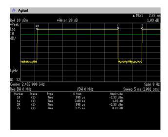
Duty Cycle = Ton / (Ton + Toff) = 2.88[ms] / (2.88[ms] + 0.87[ms]) = 76.8[%]
