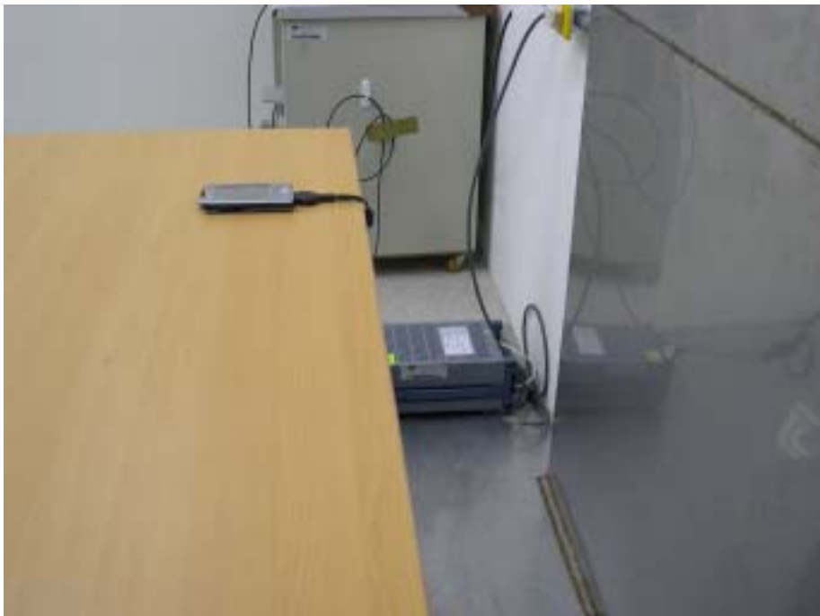
Photo 2: Conducted Emission Test Set-up
