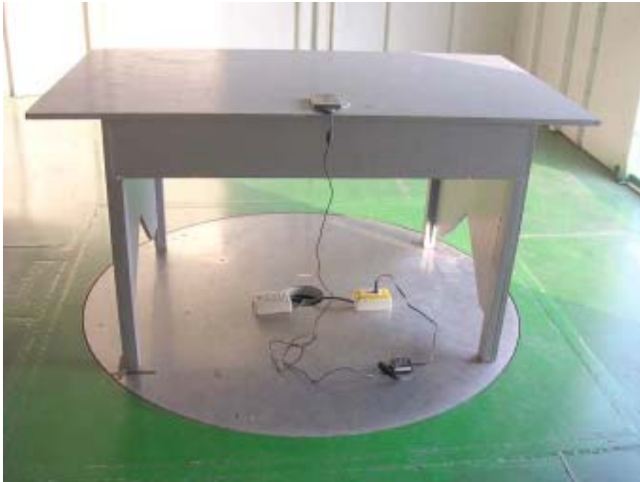
Photo 2: Radiated Emission Test Set-up
