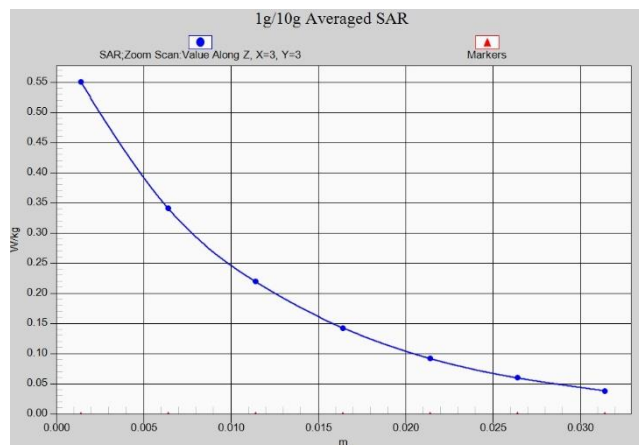
Z-Scan at power reference point (LTEB2)
