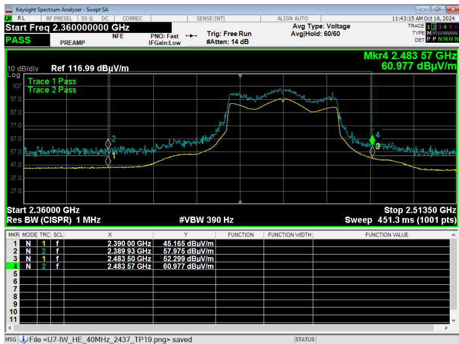
Graph 8: Radiated Upper Band Edge Plot ax 40 MHz
