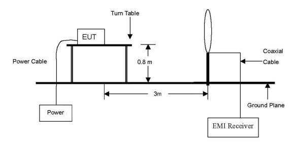
The diagram below shows the test setup that is utilized to make the measurements for emission from 30 Mb to 1 GHz.
