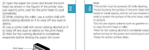
\*Do not use organic solvents such as gasoline or acetone to wipe the print head or roller. \*Wait for the rubbing alcohol to completely evaporate before turning on the power and continuing to print. \*Keep the sensor surface clean.
