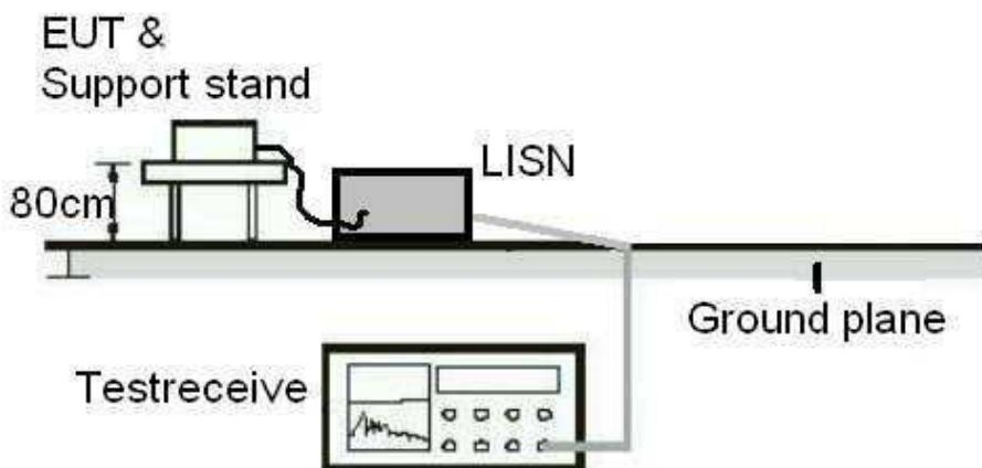
**Diagram of Measurement Equipment Configuration for Conducted Transmitter Measurement**
